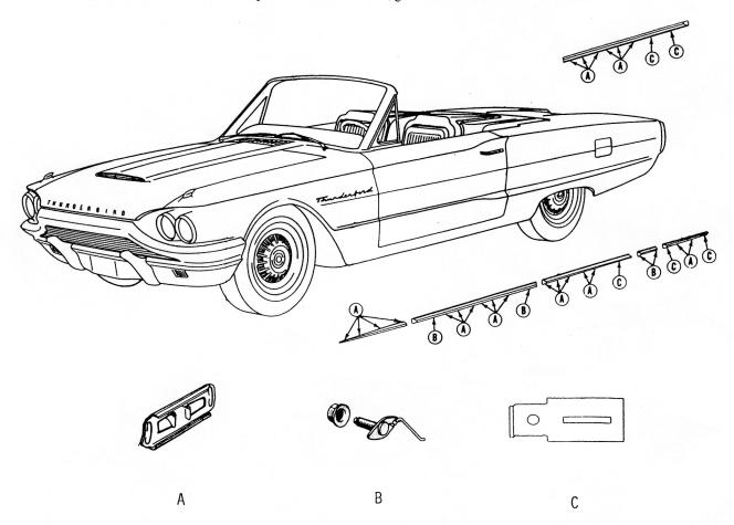
It is recommended that you mark the side of your car with a chalk line. The moldings center over the crease that runs along the side of the car. You will need a drill and drill bits to drill the holes for the clips.
